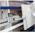
Digital dimension display for length adjustment during vertical cutting
