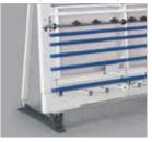
► Slatted frame automatically moves out of way to prevent saw blade cutting into rear wall slat
