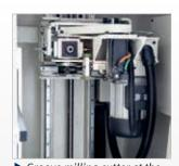
► Groove milling cutter at the bottom of the drilling unit
