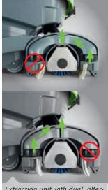
Extraction unit with dual, alternating extraction (patented). Water is taken up during forward and reverse motion
